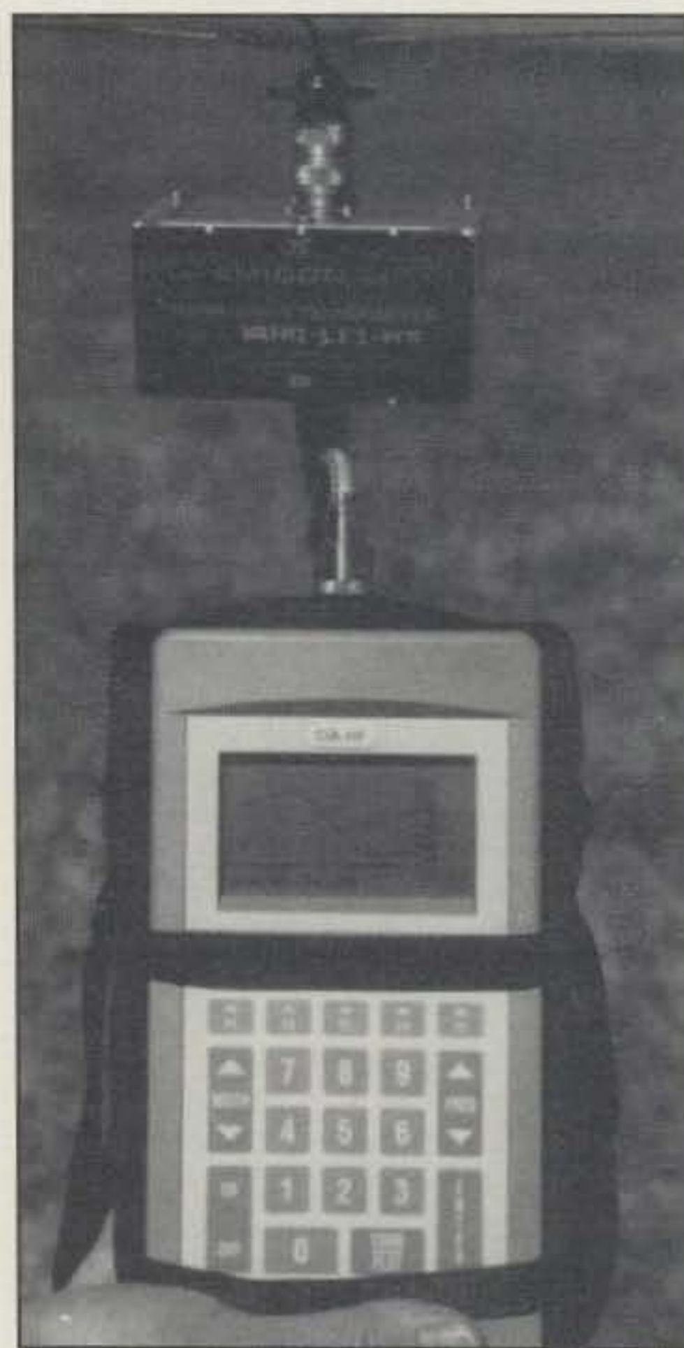
Impedance curve for European 14-element array displayed by the AEA CIA-HF Complex Impedance Analyzer and Amidon 1.5 to 1 unun transformer for matching directly to 75 ohm hardline.
